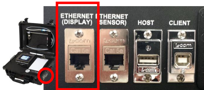
Figure 10 - Location of Ethernet port for cable connection
