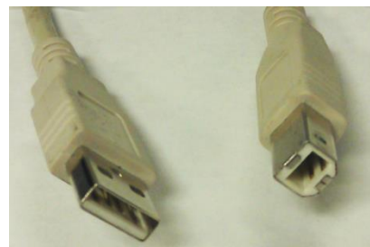
Figure 7 - USB connection types Standard-A (left), Standard-B (right)
