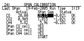
Verify span gas values to Cal Cylinder.
