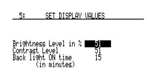
off, the instrument still operates fully, but the display is more difficult to read. To restore the backlight, press any key. To disable this function, enter  $\mathbf{0}$  and the backlight will be always on.
