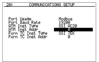
The menu page will allow the user to set up the communications settings for the PGA.
