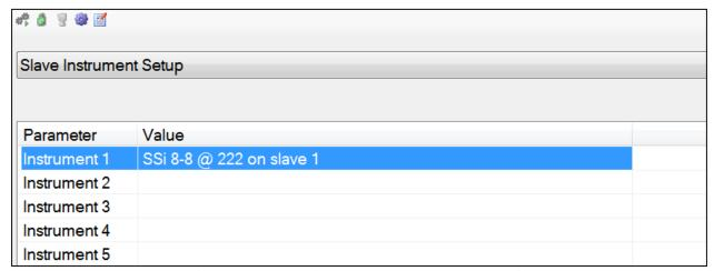
Figure 4 - Slave Instrument Setup Menu with Instrument 1 Configured
