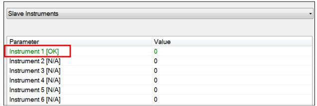
Figure 5 - "[OK]" Indication on Slave Instrument
