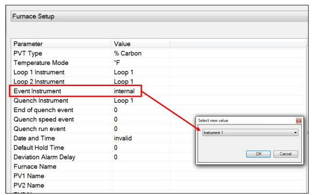
Figure 7 - Event Instrument Setup in Furnace Setup Menu
