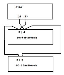
Use Slave 2 in order to make the 9015 a relay extension. Connect terminals 22 & 23 on the 9205 or 9220 to terminals 3 & 4 on the 9015.
