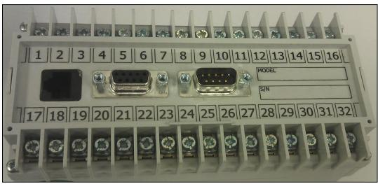
Figure 1 - Instrument Terminals
